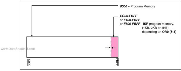
Address Space for MPC89x515A embedded Flash memory
